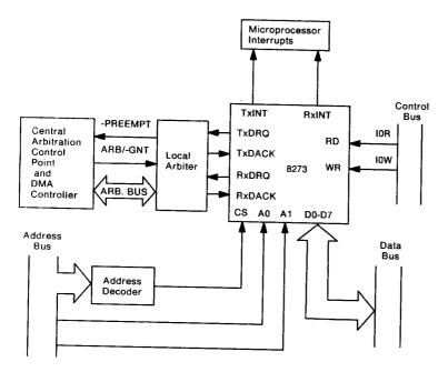
Figure 54. DMA, Interrupt-Driven System
