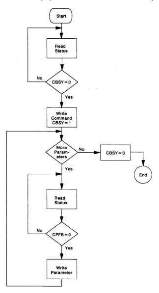
Figure 63. Command Phase Flowchart
