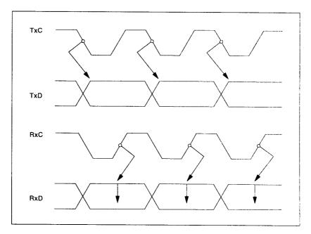
Figure 57. Transmit/Receive Timing
